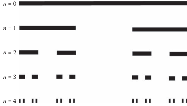
FIGURE 3.3 Construction of the Cantor set, by repeated removal of the middle third of each interval; at each step, there are two elements that are three times smaller, leading to a fractal dimension D_F = \log 2 / \log 3 = 0.631 .
